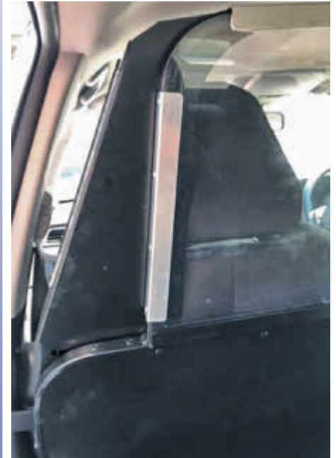
DPS screens still had gaps between the pillar that could enable a rear passenger to project bodily fluids into the front compartment.
