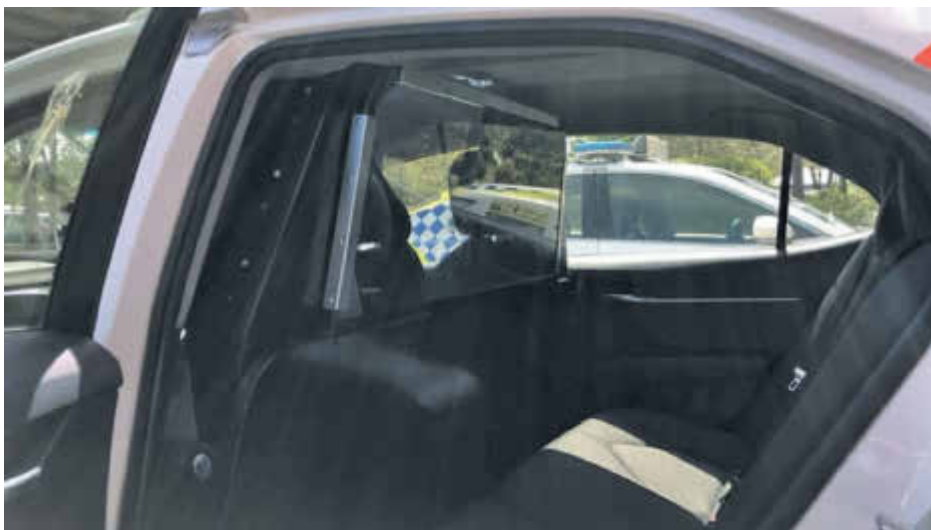
Driver Protection Screens were first installed in the early nineties in Queensland Police vehicles.
