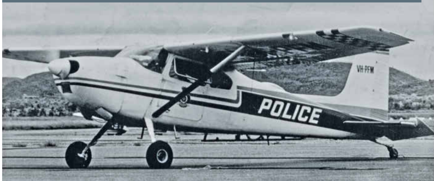
One of the two ex-Army Cessna's purchased by the QPS included larger wheels, better landing legs and reinforced wings.
